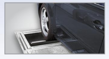
The brake tester, which forms the basic unit of the test lane, is also available with braking motors (3.7 kW motors only).
